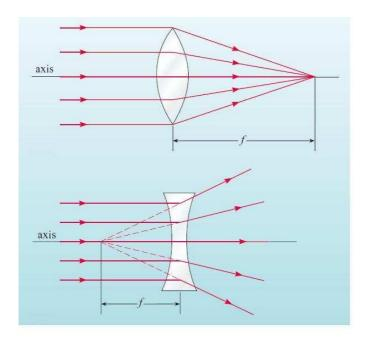
A convex lens. Parallel light rays from a distant object are brought to a focus one focal length beyond the lens. This is how the real image is formed by our objective lens.
